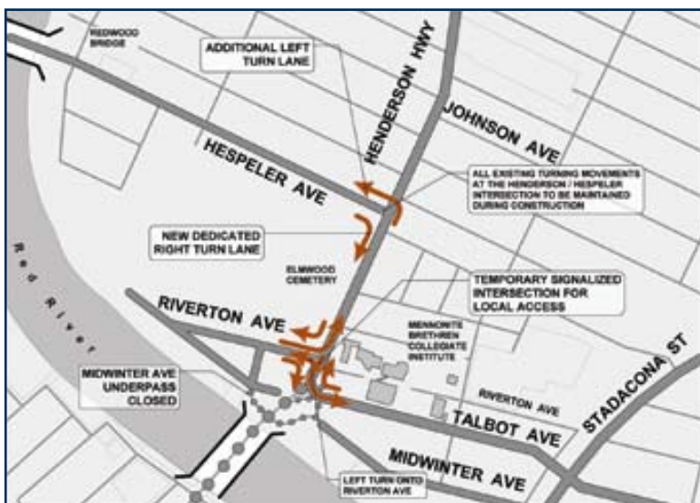
Henderson Highway and Hespeler Avenue Intersection to Talbot Avenue – new traffic flow and access
